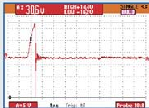
High amplitude EDM discharge pattern
