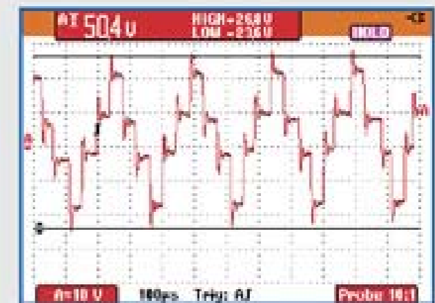
High Peak to Peak common mode voltage
