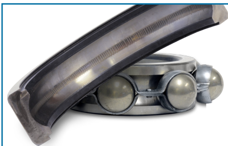
Bearing fluting, "washboard" pattern on bearing race
