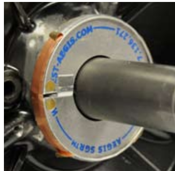
End bell with SGR installed
