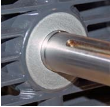
End bell with cleaned surface
