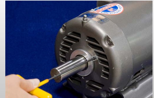
6. Secure SGR with 2 or 3 mounting clips and hardware.
