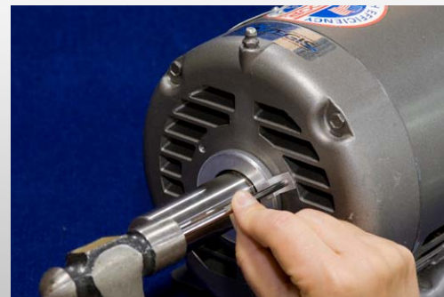
3. Mark drill point using transfer punch and mounting clip.
