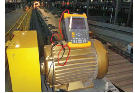
Ideal for maintenance personnel and testing contract tours, the kit can be used to test every VFD-controlled motor in an entire plant, office building, or mechanical room.
