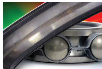
VFD-induced shaft current discharges can cause pitting (frosting) of ball bearings and fluting (the washboard pattern shown above) of bearing race.
