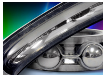
Unprotected bearing shows fluting from continual electrical discharges
