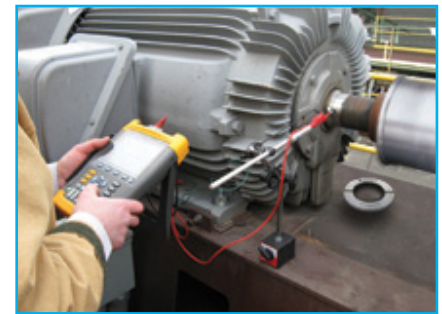
New AEGIS™ Shaft Voltage Test Kit includes a special conductive microfiber SVP probe for highly accurate measurement of motor shaft voltage levels.
