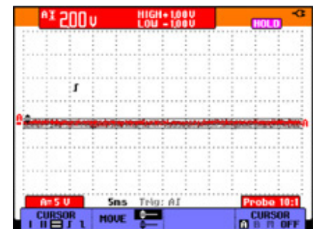
After installation of AEGIS™ rings, Reading 3 showed no damaging voltage discharges.
