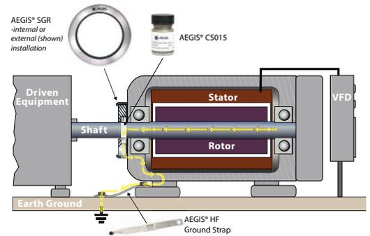
Install AEGIS® Shaft Grounding Ring – either internally or externally – on drive end or the non-drive end of motor.
