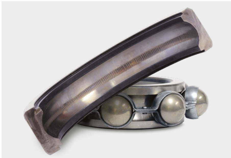
Figure 2: The “fluted” bearing race on of an electrically damaged bearing.
