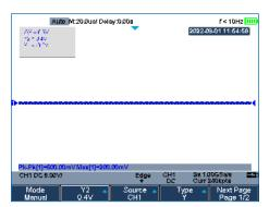
Shaft voltage reading from a VFD-driven motor with an AEGIS® Bearing Protection Ring
