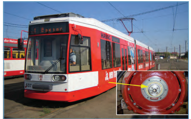
Figure 1: This all-electric tram in Halle (Saale), Germany, suffered bearing damage from inverter-induced voltages until the problem was solved in 2007 with the installation of an AEGIS® SGR Bearing Protection Ring (inset) on the shaft of every traction motor in the fleet. The city has had an electric tram system since 1891.
