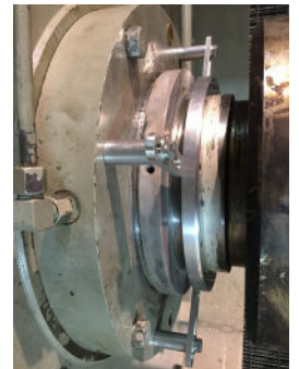
AEGIS® PRO installed with PRO Brackets
