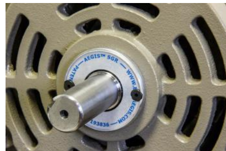
External Installation on Motor Bracket
