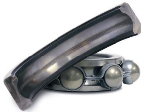
Bearing without protection: severe fluting damage or severe electrical damage
