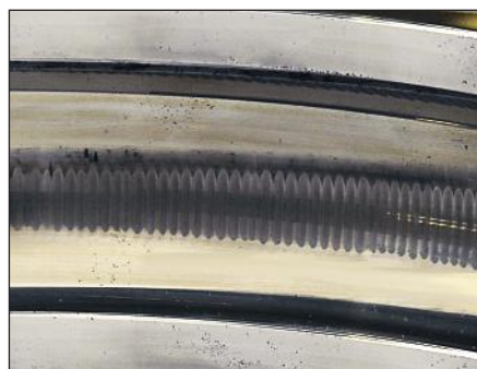
Bearing with fluting formation.
