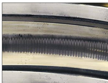
Bearing with fluting formation.
