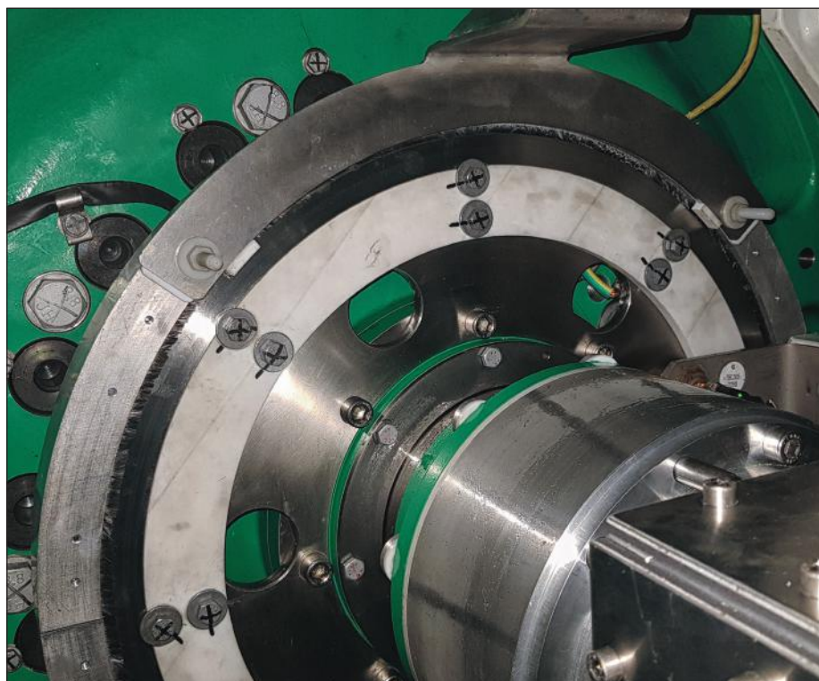
After installing the AEGIS® PRO ring, the shaft voltage could be reduced to less than one volt.
