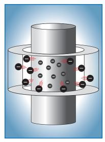
Field emission is a form of quantum tunneling whereby electrons move through a barrier in the presence of a high electric field. It provides grounding across gaps of 2 nm to 5 µm. The electric field from the shaft voltages creates the conditions for the AEGIS® ring fibers to take advantage of field emission electron transfer from the shaft.
