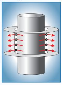
This mechanism is based on the ability of electrons to "tunnel" across an insulating barrier, and works for gaps smaller than 2 nm.
