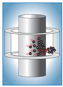
This process results from the cascading effect of secondary electrons released by collisions and the impact ionization of gas ions accelerating across gaps greater than 5 µm. This ionization creates negative and positive ions which neutralize the shaft voltage.
