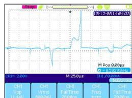
Amplitude will need to be adjusted according to the conditions. Set to show complete wave from top peak to bottom peak using the scale buttons.
