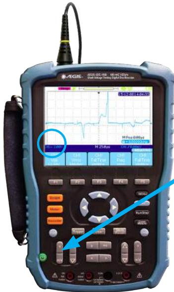
An EDM discharge pattern will show a climb in voltage and then a sharp vertical line. The sharp vertical line shows the moment of discharge to ground. To get a good image of a discharge, you may need to adjust the display scale.
