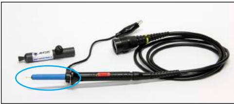
1. The AEGIS® Meter probe has an insulated sleeve over the tip. Do not remove this cover.
