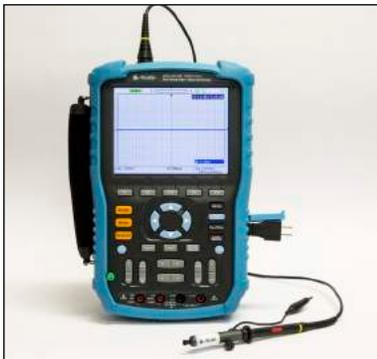
Now the scope is set up to calibrate the probe. The AEGIS-OSC-9100 includes a two-pronged calibration dongle that plugs into the side of the scope. This micro-USB dongle generates a square wave used to fine-tune the probe.
