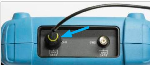
4. Connect 10:1 probe into Ch 1.
