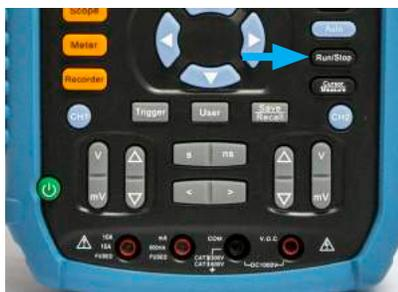
While making measurements, **RUN/STOP** freezes the screen. When stopped, the word **STOP** will appear in the upper left of the screen.
