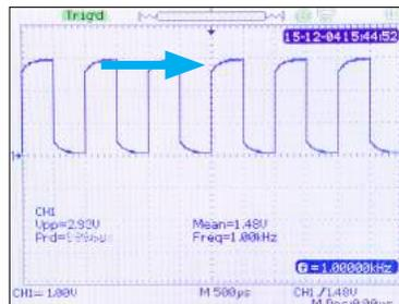
Press **AUTO**. The scope will display a train of approximately square waves of amplitude 3V and frequency 1 kHz.
