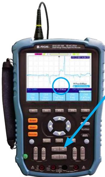
Control the horizontal scale of the displayed signal by adjusting the time scale. 500µs (microseconds) is a good place to start and then adjust the time based on the conditions. The selected seconds per division setting is shown at the bottom center of the screen. The EDM wave forms are best displayed at a setting of 50µs/div or less. Adjust the time setting to show the desired waveform.
