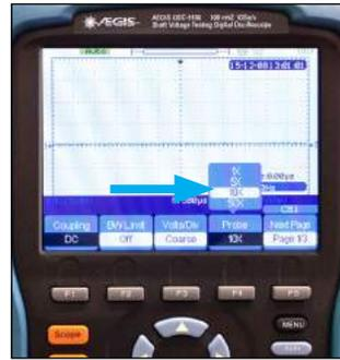
Select **10X** with the blue up and down arrows and press **ENTER**. Press **MENU** to exit the **CH1** menu.
