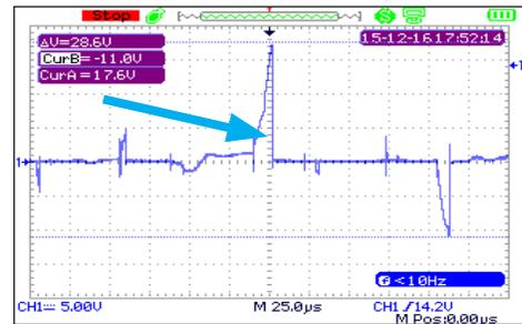
The voltage measurement of 28.6V peak to peak is an example of the voltage discharging through the bearings without AEGIS® shaft grounding.
