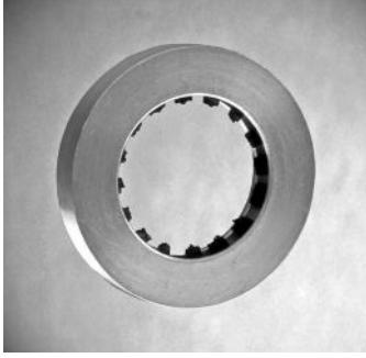
Fig. 6. Conductive microfibers assembled in rings to form static charge dissipation devices for mitigation of EDM-bearing currents.
